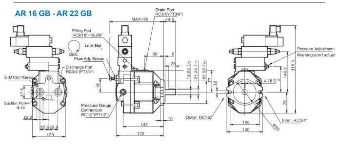
Note: - Inlet - Outlet port are for standard rotation (clockwise)
