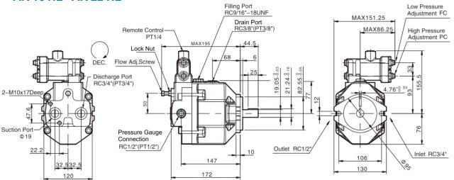
Note: - Inlet - Outlet port are for standard rotation (clockwise)
